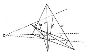
Let O be the centre of perspective of the given triangles, then the lines joining the points bc, ca, ab to the points b'c', c'a', a'b'intersect in O.
